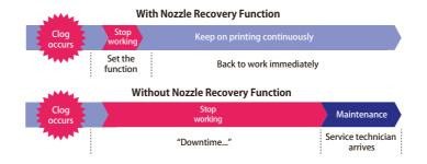
When print troubles occurred due to clogged nozzle and when the nozzle cleaning does not work, the conventional printer have to stop printing and wait for the arrival of service person. With Nozzle Recovery Function, the continuous printing is possible by recovering the image quality without slowing down the speed even if a nozzle is removed or taken away.
