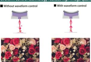
Mimaki's unique advanced ink droplet ejection control makes it possible to eject ink droplets that are close to perfect circles and accurately land on media. By improving landing precision, edges, characters, ruled lines can be expressed sharply.
