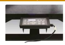
The control panel is in front and at the rear of the main unit. Work efficiency is improved as there is no need to move to the front or the real of the unit to operate it.
